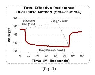
The typical effective resistances of fresh Energizer alkaline cylindrical batteries (using a 5 mA stabilization drain followed by a 505 mA 100 millisecond pulse) will be approximately 150 to 300 milliohms, depending on size.
