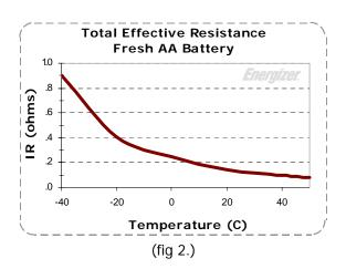
In summary, internal resistance can be calculated based on the voltage drop of the battery under a known load. Results will be affected by technique, settings and environmental conditions. The internal resistance of a battery should be viewed as a general guideline and not as a precise value when applying it to the expected voltage drop in a specific application.
