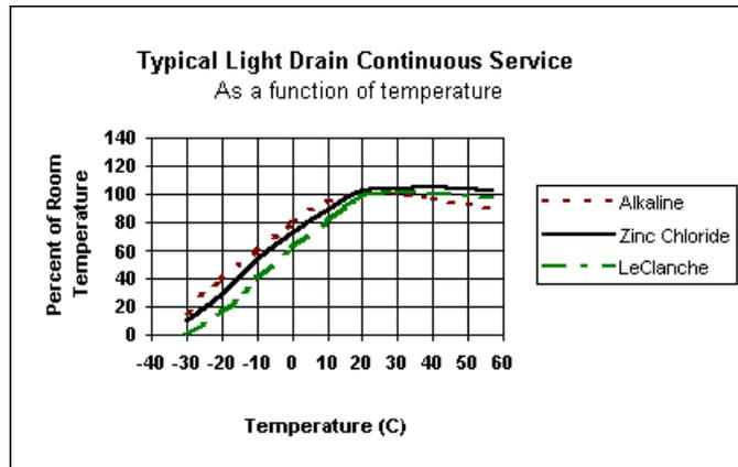
**Light Drain** is defined as a current that would discharge the battery after 50 or more hours of use at room temperature.
