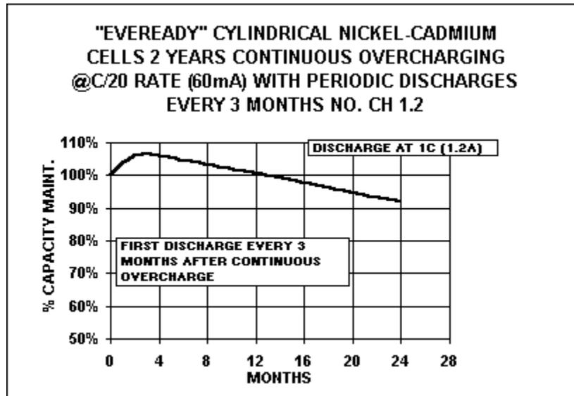
The chart above illustrates maintenance vs. months of continuous overcharge at the 20 hour rate with periodic discharges every 3 months at the 1 hour rate. The cells maintain 90% of their initial capacity after 2 years of this overcharge regimen. This pattern of use would occur if batteries are left on charge continuously and used one cycle only on an occasional basis.
