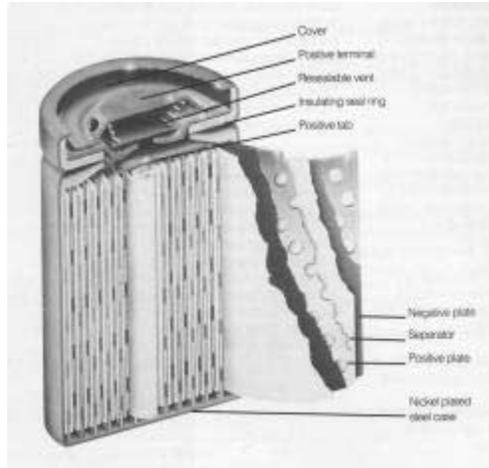
Sealed nickel-cadmium cells under certain abuse conditions such as excessive charge or overcharge rate, deep discharge with subsequent polarity reversal, may develop high internal gas pressure. Usually the gas is oxygen, although hydrogen is also evolved in some cases. Either or both hydrogen and oxygen must be vented.
