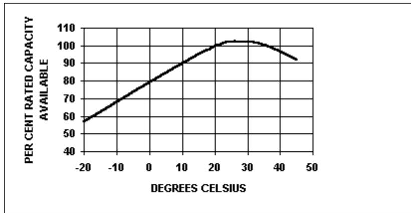
Charging nickel cadmium cells below the recommended temperature can cause oxygen pressure build up and activation of the resealable safety vent. Multiple vent activations will reduce cell capacity.
