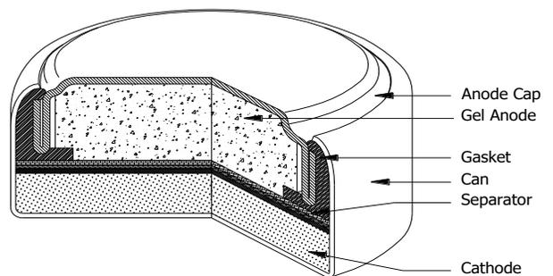
DESIGNED FOR USE ON CONTINUOUS LOW DRAIN
