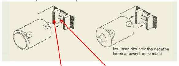
The distance between the plastic rib and the battery contact needs to be <u>less than</u> 1 mm.
